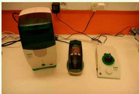
The Experion™ system (Left to right): electrophoresis station, priming station and vortex
